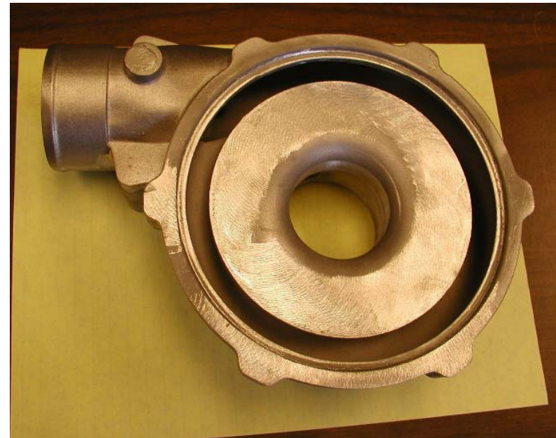
Aluminum Pump Housing Rapid Prototype Casting
