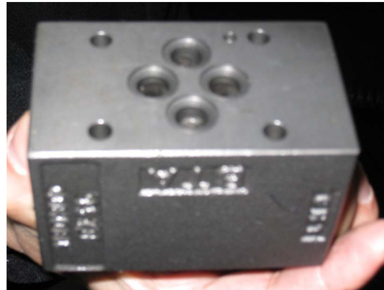
Finished D1VW Valve Casting, Cast and Finished Machined at Foundry
