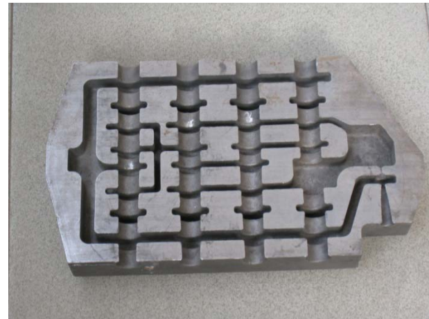
Cut Away of 4 Spool Valve Body
